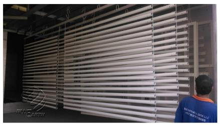
crosslinking, requires a certain temperature for a certain length of time in order to reach full cure and establish the full film properties for which the material was designed. Normally the powders cure at 200°C (390°F) for 10 minutes. The curing schedule could vary according to the manufacturer's specifications. The application of energy to the product to be cured can be accomplished by convectional curing ovens.
